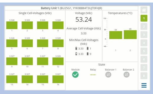
A battery module contains two battery blocks with each eight cells. The more detailed view into the single Battery Modules allows a closer look at each cell, its voltage and the temperature of each Battery block.
